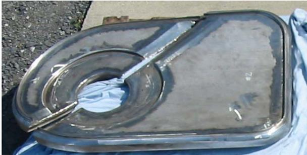
**As-Constructed Split PMCap (Underside View)**
