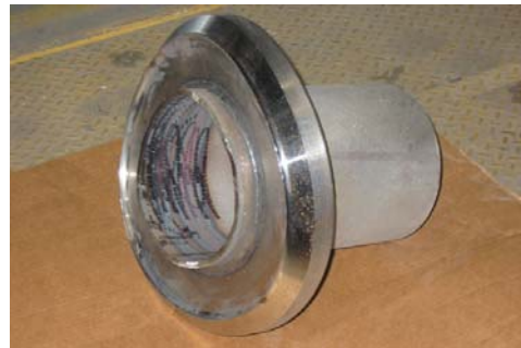
8" PMCap-Nozzle – Carbon Steel PMCap , CrMo Nozzle, and 304 SS Liner
