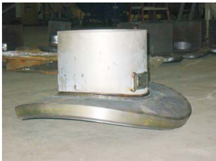
16" PMCap-Nozzle - Carbon Steel PMCap , 304 SS Nozzle, and 304 SS Liner
