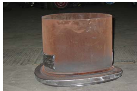
24" PMCap-Nozzle – Carbon Steel PMCap CrMo Nozzle, and 304 SS Liner
